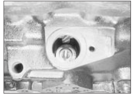
6.8 Correct position of oil pump driveshaft prior to fitting distributor
